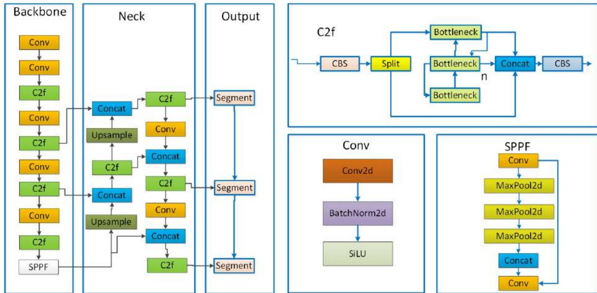
Figure 1. YOLOv8 network model structure diagram
