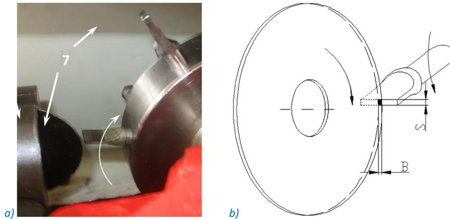
Fig. 3. Image (a) and diagram (b) of the interaction of the sample and the disc counterbody during the contact fatigue test.
