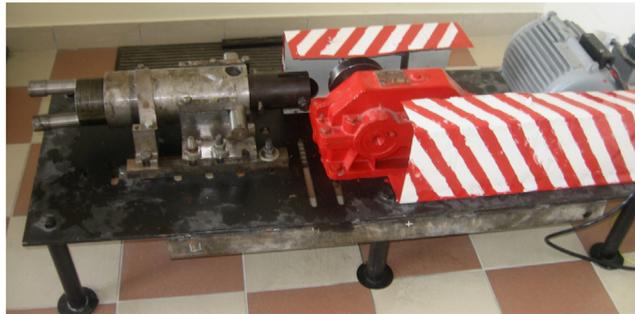
Fig. 2. General view of the contact fatigue testing facility.
