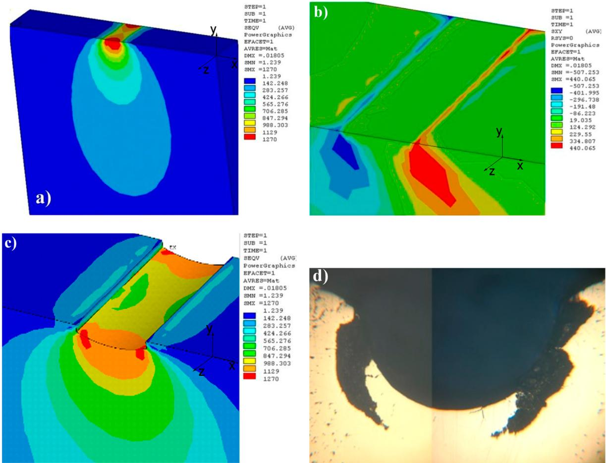
Fig. 5. Distribution of equivalent (a) and tangential (b) stresses over the working surface of the sample at the initial moment of testing, equivalent stresses at a hole depth of 0.2 mm (c) and the pattern of crack propagation in the experimental sample (d).
