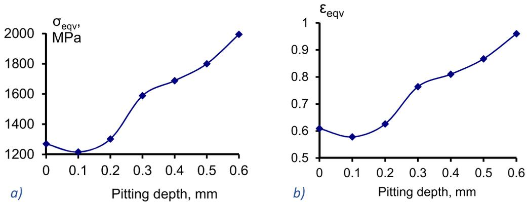
Fig. 7. Change of equivalent stresses (a) and strains (b) in the lateral plane of the working part depending on the pitting depth.
