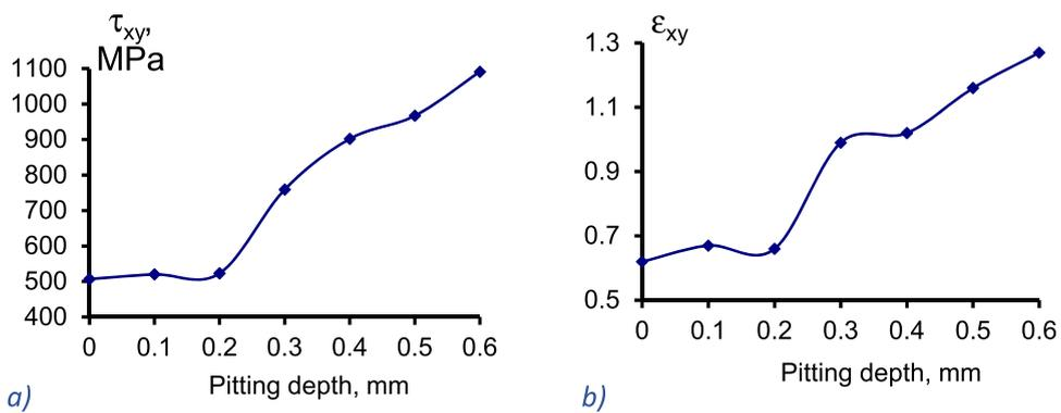
Fig. 6. Change of tangential stresses (a) and shear strains (b) in the lateral plane of the working part depending on the pitting depth.
