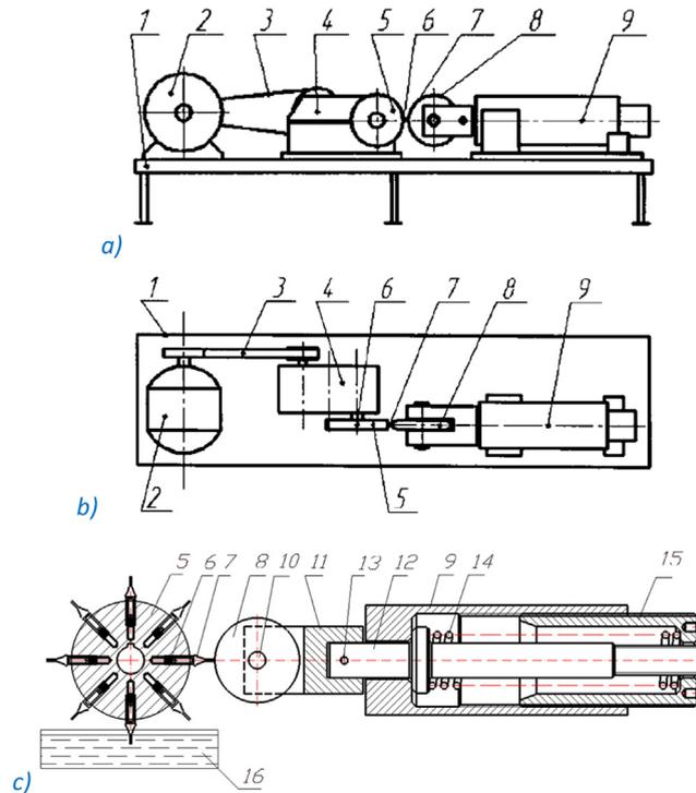
Fig. 1. Device for testing materials for contact fatigue and wear: a – front view; b – top view; c – loading unit for experimental samples.
