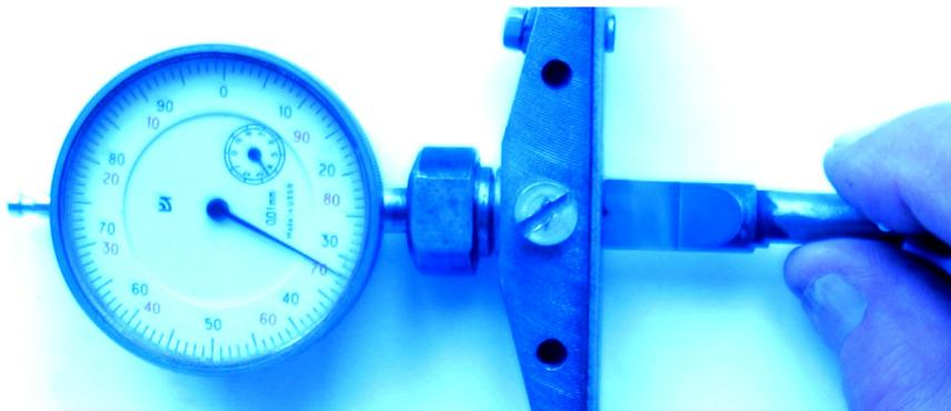
Fig. 4. Direct measurement of the pitting depth.
