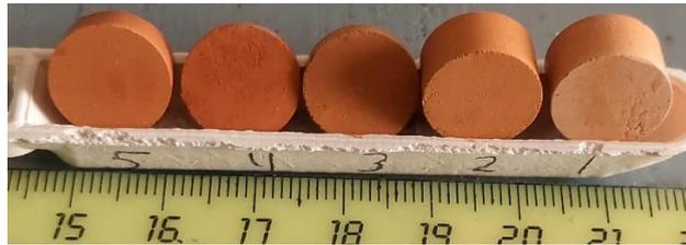
Figure 2 – Photo of tableted targets annealed in air at  $T=700\text{ }^{\circ}\text{C}$  (1 hour)
